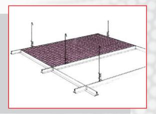
Most Louverlux aluminum louvers can be seamlessly suspended. This means that no T-bars or cross-bars are visible. In this case the panels have all around half ends and are fixed to each other with connection clips.
